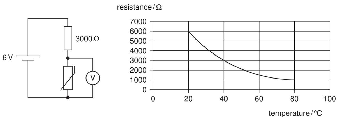
What is the temperature of the thermistor when the voltmeter reads 2 V?
